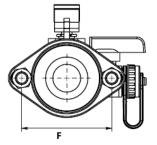
**Specifications:** Designed for residential, commercial or industrial use with water only. This approved Webstone valve is actuated by a blowout proof stem and features an adjustable packing gland. HV models fit both standard and high velocity pumps.
